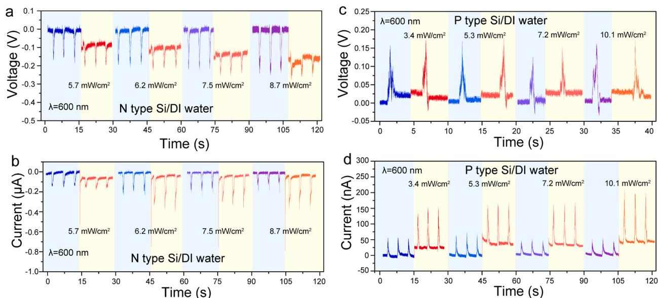
**Fig. 3.** Effect of light intensity on the coupling interaction between photovoltaic effect and tribovoltaic effect. The effect of light intensity on the (a) tribo-voltage, (b) tribo-current between the DI water and the N-type Si. The effect of light intensity on the (c) tribo-voltage, (d) tribo-current between the DI water and the P-type Si.
