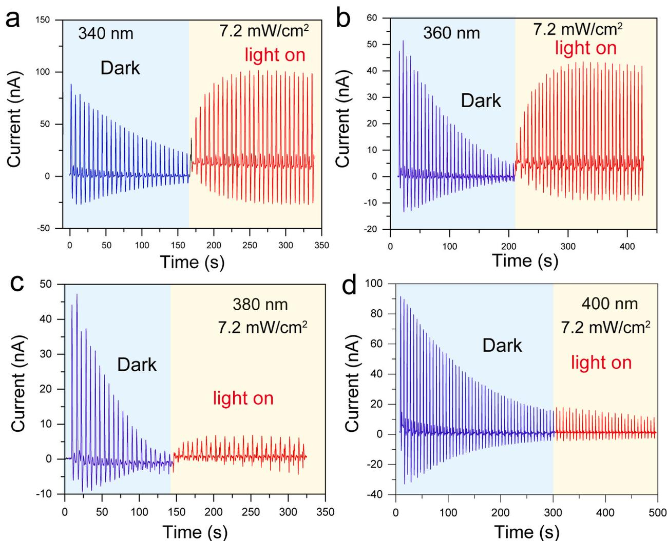
**Fig. 4.** The coupling of photovoltaic effect and tribovoltaic effect at the DI water and the  $\text{TiO}_2$  interface. The oscillogram of the short-circuit current when a DI water droplet slides on a  $\text{TiO}_2$  surface in the dark condition and under light irradiation with (a) 340 nm, (b) 360 nm, (c) 380 nm, (d) 400 nm light wavelength,  $7.2 \text{ mW/cm}^2$  light intensity.
